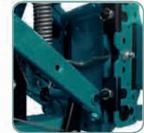
Hook Planting unit lifting device.
